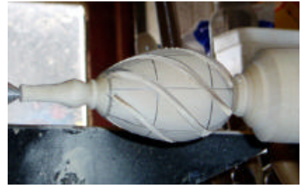
Stages in making a spiral finial. Marking up (above), cutting with arbortek, (left and right and almost done, (below)
