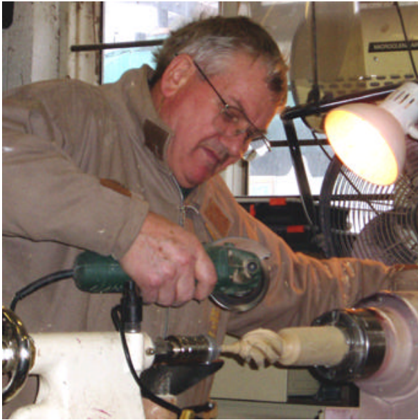
Stages in making a spiral finial. Marking up (above), cutting with arbortek, (left and right and almost done, (below)
