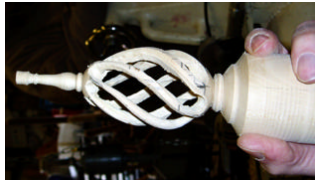
Stages in making a spiral finial. Marking up (above), cutting with arbortek, (left and right and almost done, (below)
