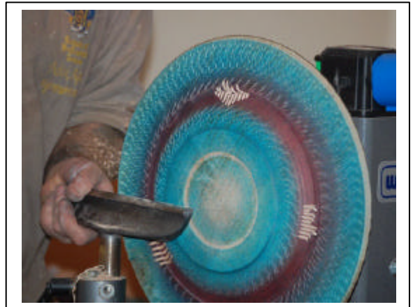
20 Right Different carved patterns. Note waste fibres from carving not yet cut off. This is done afterwards to achieve better finish to the ends of carved grooves.
