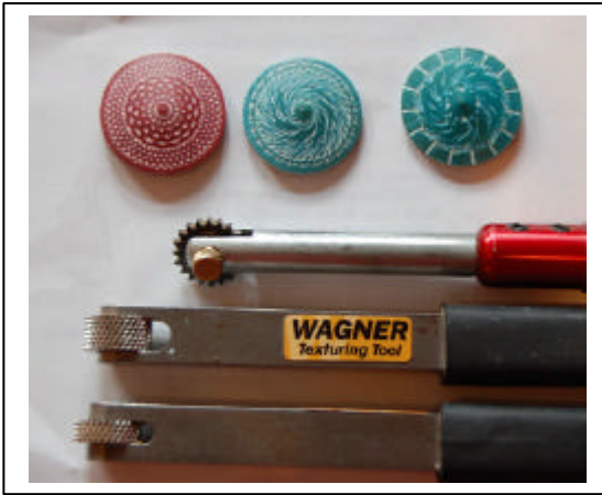
15 Left Textures on end grain discs from small Sorby & 2 Wagner tools.
