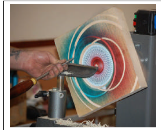
12 Right Re-mounted on new centres and cutting more grooves.
