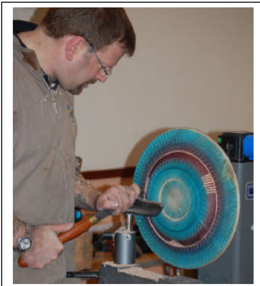
21 Left & 22 Right Cutting ring to terminate carved grooves cleanly.
