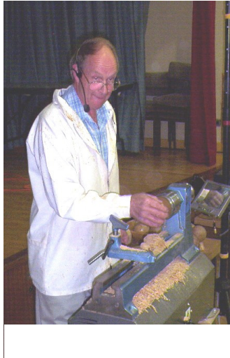
Picture 2 : Using the 'cup pattern' Adrian sands and polishes the ball which now spins freely in the cup like a bearing
