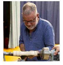
the skew over the lines to form the beads, by cutting away the unwanted stock.
