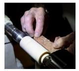
piece of plywood that had both a diagram and the measurements of the shape that he wished to reproduce multiple times. There were also sharpened panel pins that marked the prominent points of the design protruding
