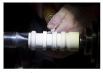
The shape was formed by using your choice of gouge, always using the bevel, and turning down into the wood rather than upwards as this can split the fibres and give
