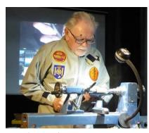
'slightly larger' than the diameter of the mandrel bushes. He then reduced this to the correct diameter using 240 grit sandpaper with the lathe turning, then stopped the lathe and
