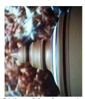
the 'wings' of the square Corian block and turned it to round and blended in the Corian to the shape that he desires for the lid of the finial. This was then sanded to suit and finished off with some 0000-steel wire wool and Chestnut friction polish. Gary used three coats of
