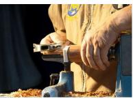
shoulder was perfectly square, until it was a tight fit. Gary applied a bit of super glue and a spray of accelerator and tapped the Corian onto the piece to ensure a completely perfect fit as he 'on-laid' it onto the piece.
