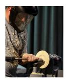
Tom then blended in both sides of the platter with push cuts to quickly remove stock, and then the mortice, followed by a quick sanding with the power sander on the front, inside and the back.
