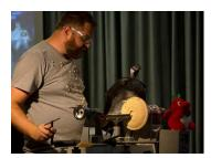
important to keep the tools sharp as pine doesn't like being 'scraped', it likes to be cut. He then placed a Forstner (the same size as the chuck) bit into the tail stock and bored the mortice
