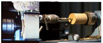
the drill bit into the Jacobs Chuck and started to drill a hole through the piece. When he had drilled the hole a few millimetres deep, he stopped using the winder on the tailstock to force the drill bit into the wood, instead he continued to 'manually' push the drill into the wood by unlocking the tail stock and forcing it towards the Chuck to required depth.
