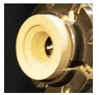
The base is then 'reverse turned' by hollowing out the piece still left in the chuck to the diameter of the circumference of the base, which is then inserted into it, thus creating a jam-chuck. To get rid of the nipple, just sand it off and put some
