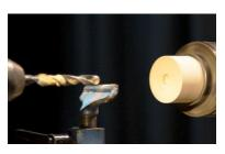
drill bit. He drilled a hole the same diameter as the spigot using the same 'push the tail stock end' method to the correct depth for his needs.
