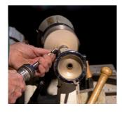
the intention of making a 'chucking' point at the tailstock end.
