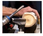
This is quite a tricky thing to do as the cutting edge of the gouge will be mostly going 'through air' as the points rotate and they will only very briefly come into contact with the wooden points as they
