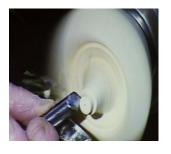
With the tool handle down, he started to create the inner profile of the piece by removing stock from the inside. Again, this needs to be done carefully as the tip of the tool tends to want to be thrown outwards, this is countered by adjusting the angle that the bevel is contacting the wood.
