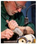
Mike then removed the piece from the chuck and created a small MDF jam chuck and reverse mounted to give access to the base. The trick is to centralise the piece onto the jam chuck and another homemade revolving centre on the tailstock end,
