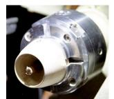
especially created for the same diameter ball, this is basically a hollowed out blank of a slightly smaller diameter that has a hole bored straight through its length that will accept the chuck ram rod. The sphere is then pressed
