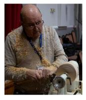
and a live centre for safety and turned to the same 4mm base size as the hole he'd drilled into the top of the pear. When he was happy with the shape, he parted it from the blank and did an angled cut with a sharp Stanley type knife to replicate the cut end of the stalk, which is then inserted into the drilled
