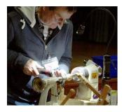
ram rod towards the sphere causing it to push away from the chuck, the sandpaper hand pushes it back into the jamchuck causing another part of the sphere to be in contact with the sandpaper and smooth it all out. This process
