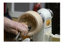
The bowl was the hollowed out using a small gouge.
