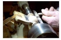
With the sphere completed Mike then had to remove the two supporting lugs that were left by parting them off closely to the edge of the sphere.
