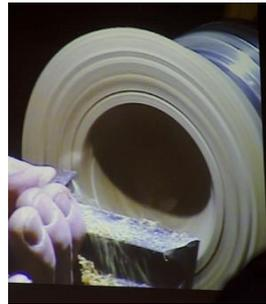
He then changed to a negative scraper to finely adjust the shape. When he had finished off the shape to his satisfaction, he removed it from the chuck and rotated it to commence the hollowing.
