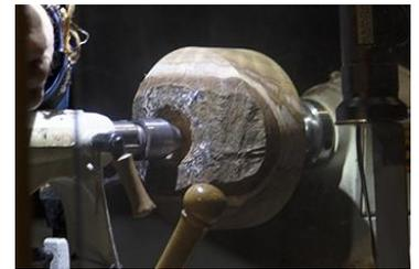
To do this it Mike told us that he uses the edge of the tool rest as a visual guide to indicate how close the centre line of the bowl is when the piece is rotated on the lath by hand, if the piece is not aligned accurately, it may be necessary to 'tap' one side of the blank to help align it, then rotate the bowl and check again.
