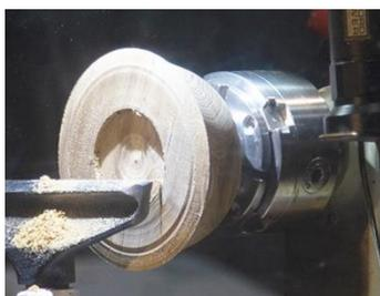
When the recess has been created, Mike turns the bowl and attaches it to the chuck ready to shape the outside of the bowl, he also completely removed the tailstock from the lathe to allow total access to the bowl, this enables it to be turned without any danger of the handle of the gouges getting
