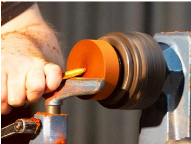
Fig 24 – Cleaning the end of the lid
