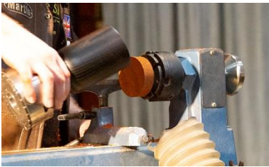
Fig 23 – Testing the fit of the lid to vessel
