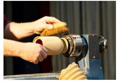
Fig 20 – Wire brushing the outside
