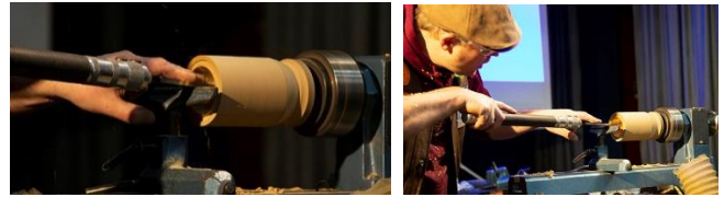
Fig 9 and 10 – Scraping the inside
