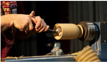
Fig 15 – Sanding the inside
