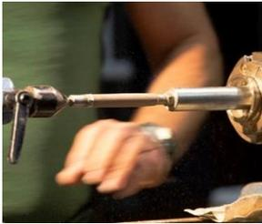
Both the Abranet and the Nyweb pads are best used on the lower surface of the workpiece, so that your hand does not obstruct your view.
