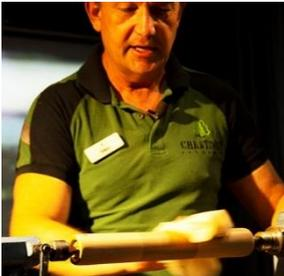
grit, but then remove as much of the sanding dust with a Chestnut **TAC CLOTH**. This is a cloth that has been impregnated with a resin that will 'pick up' the remaining dust from the surface and
