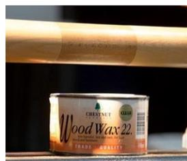
of Bees wax and Carnauba wax, which is best used in solid form rather than hot or runny. It is used by rubbing it onto the piece until it begins to offer resistance, then turn
