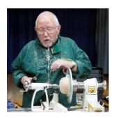
When he was happy with the overall shape and thickness Richard removed it from the chuck and attached it to a set of buttonjaws. He made sure that the bowl was firmly held by the button-jaws but taking care not to over tighten it and crack the walls of the bowl.
