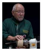
tenon a slight undercut in order for the jaws to securely grip the workpiece when it was reversed and held in the jaws.
