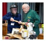
With the tenon completed Richard removed the piece from the pro-drive and attached the tenon to the chuck, then trued up the piece. Richard then drilled a hole through the length of the piece to a depth and diameter that
