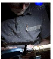
pointed out that the safest way to make the finial is to "work backwards" by starting from the tail stock end to form the top point of the finial. This ensures that there is still strength in the piece as it is being shaped and thinned, as the shaft and any embellishments are created.
