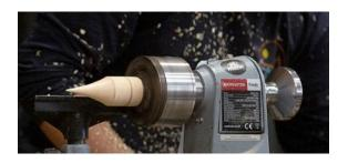
He said not to make it too fine. He then used a parting tool to remove wood near the chuck end and provide some clearance.
