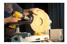
Tom then reversed the wood and faces off using a push cut and then a sheer cut. He then took the sharp edges off the edge of the piece.
