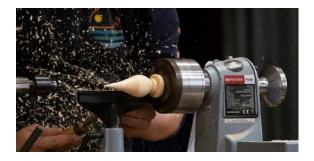
He then did a finishing cut and then sanded through the grits, he mentioned the importance of good extraction when sanding, as he did not have suitable extraction for the demonstration he kept his sanding to a minimum.
