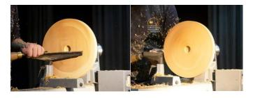
He then used a hand made jig, made from an old pillar drill stand. He used this with the index system to drill out holes for coins at the clock positions.
