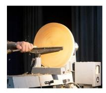
Part way through the demo Tom showed his home-made sharpening jig and with this, and a CBN grinding wheel, he sharpened the bowl gouge for a finishing cut. He then used a negative rake scraper and checked the face was square with a ruler.
