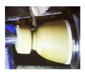
tight fit inside the hollowed-out middle, Mike then inserted a piece of tissue paper between both faces and applied the tailstock, this was then tightened so that the point of the centre made a small indent to ensure that the piece was held tightly so that the stem could be worked on and shaped to an elegant design.
