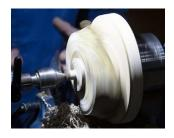
the blank on the jam-chuck so that stock would be removed from the piece equally from both sides, this ensures that the grain pattern remains similar on both sides. As it was attached via the jam-chuck Mike could ease the tail stock pressure and slightly adjust the position of the piece to ensure that he was removing stock from where he intended.
