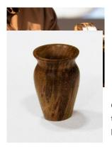
The vase was parted off with an angled cut as before, to undercut the base. The importance of measuring the drill depth was illustrated as the finished piece had a hole in the bottom!
