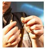
A special hollowing tool was then used to hollow out the inside. To prevent the tool from kicking while hollowing, the handle was held under the right arm.
