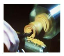
As before, the vase was then partially parted off before sanding (in this case starting at 180 grit). Sanding by hand with the grain can remove sanding rings. For wooden pieces Anna-Marie sands to 400 grit, though for acrylic, corian etc she would use finer grits. This time the piece was finished with sanding sealer, lightly sanded and then microcrystalline wax was applied with the lathe stopped, then buffed with the lathe running.
