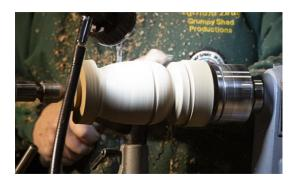
When the piece has been rounded off Richard then faced off the edges and created a Tenon on either end that was a suitable size to be safely held in the chuck. For this measurement Richard set his callipers to 54mm, to suite his chuck and cut the Tenon to that size and slightly tapered the inside to give a better grip to the jaws of the chuck.
