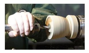
Again, Richard inserted the drill into the Jacobs Chuck and drilled a small hole to start the hollowing process, he continued to drill into the piece but making sure that the hole was not too deep. He then removed the Tailstock and adjusted the tool rest to allow for the Simon Hope boring tool to reach the inside, he then started to remove stock from the inside and create the shape that he wanted to achieve.
