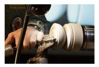
Richard then started to hollow out the bottom section by making a small groove near the rim, he explained that this prevents any accidental tool slippage that may damage the outside edge of the rim. Richard then inserted a drill into his Jacobs Chuck which he then placed into the tailstock end and with the lathe at a medium speed he started to bore a hole into the centre of the base of the egg, making sure not to go too deep.
