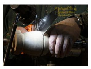
Due to the splits in the wood on the bottom section, Richard removed wood to suite the deficiencies in the blank. By using a smaller gouge Richard created a tight curve for the base of the egg and its pedestal. Then by using a thin parting tool
